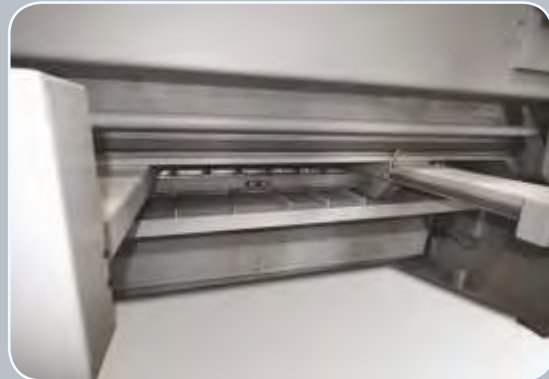
Position 1: Thanks to the RSS System, the sheet-metal is supported on the back gauge and does not bend.
